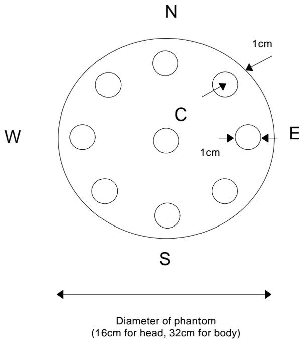
**Figure 14. Chamber Positions in the CTDI phantoms.**
