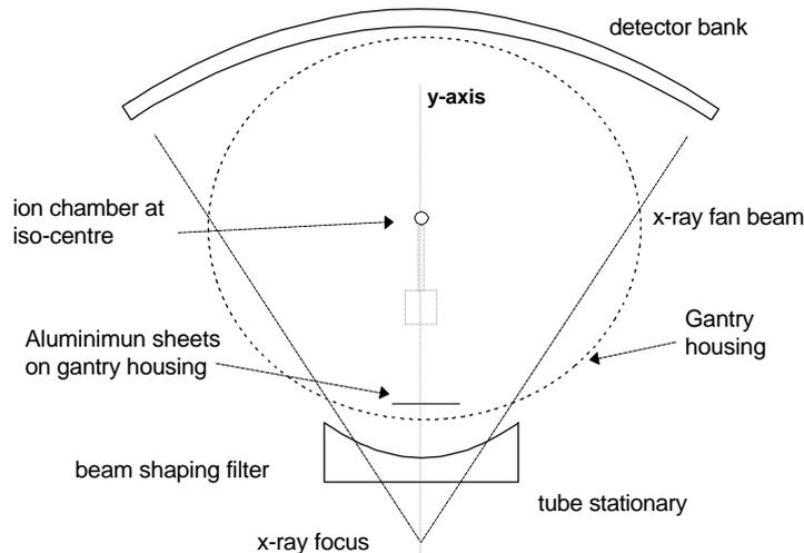
**Figure 10. Schematic diagram for HVL measurement.**
