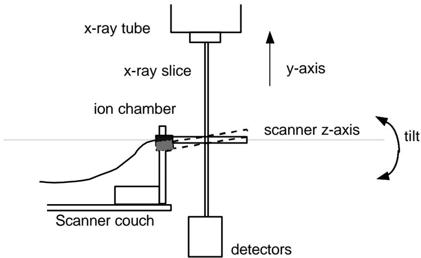
**Figure 15. Chamber Tilt, Lateral View.**
