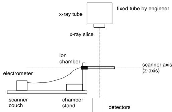
Figure 8. Chamber overhanging the table end.
