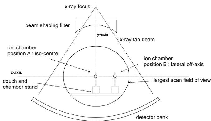
**Figure 9. Showing transaxial off-axis positioning of the chamber.**
