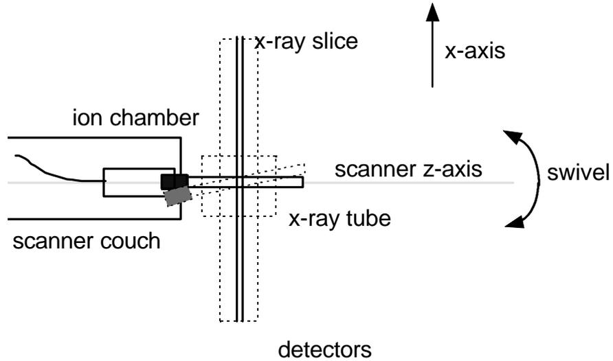
**Figure 16. Chamber Swivel, Plan View.**
