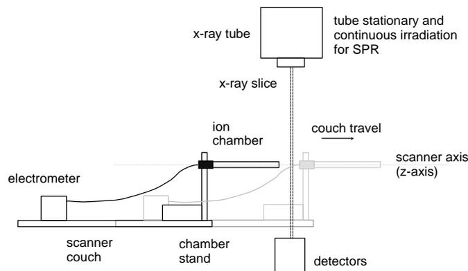
**Figure 7. SPR : couch top direction of motion.**
